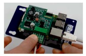
RS232 serial connection to the control panel with a terminal block.
